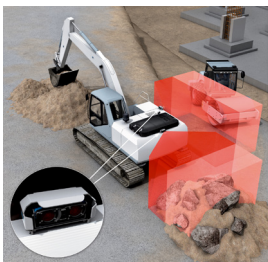
Stereo for active collision warning in harsh outdoor environments
